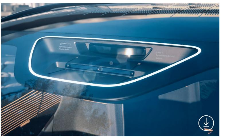
In the upper area at the front there is a lidar and camera sensor unit: the Centre Pilot
