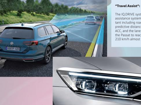
The IQ.DRIVE system combines all of the assistance systems: the traffic jam assistant including roadworks assistant, the predictive distance-regulating assistant ACC, and the lane assistant. This allows the Passat to reach speeds of up to 210 km/h almost entirely automatically.
