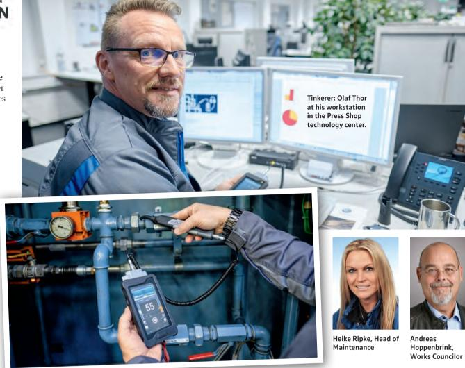
Measurement: Leaking air can be detected with a digital ultrasound device.
