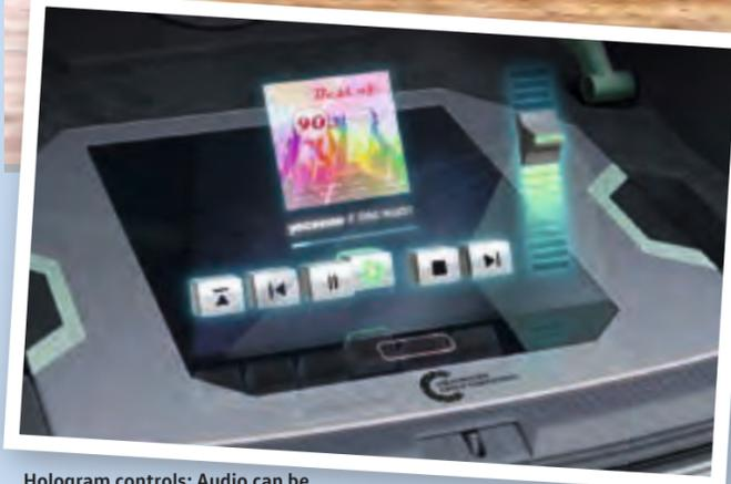
Hologram controls: Audio can be controlled via floating buttons.
