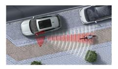
If another road user is approaching from behind as an occupant is exiting the vehicle, the exit warning system can issue warnings in various stages.
