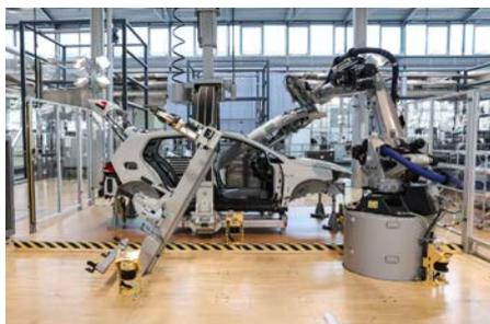
World first: The headliner for the e-Golf is now being fitted by a robot as standard.
