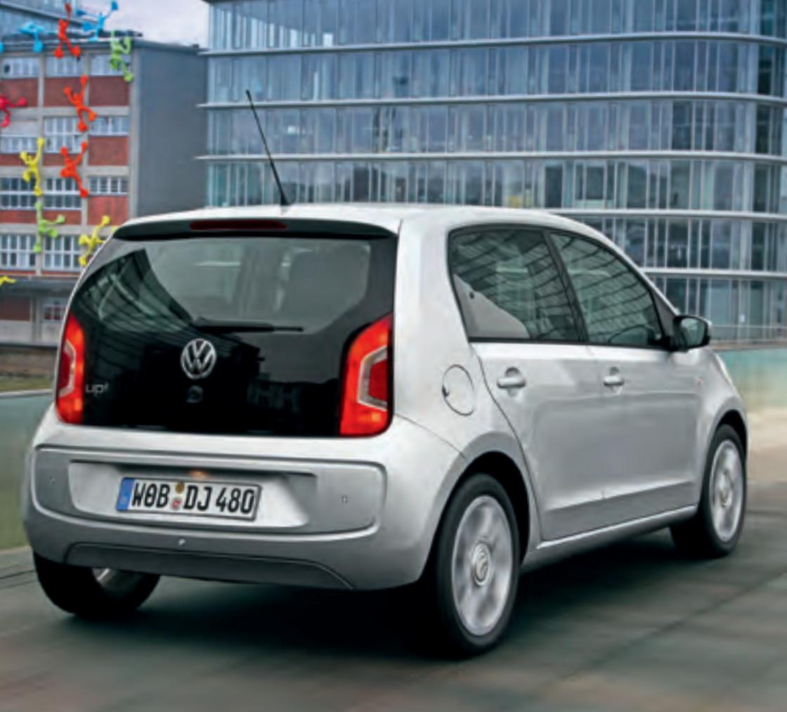
**Wolfsburg / Bensberg, March 2012.** At 3.54 m in length and 1.64 m in width (without door mirrors), the up! is one of the smallest of four-seat cars. The Volkswagen is 1.48 m tall. These dimensions are identical for both body versions of the up!. Its overall length consists of remarkably short body overhangs and a very long wheelbase (2.42 metres) – a body layout that fully utilises the available enclosed space.
