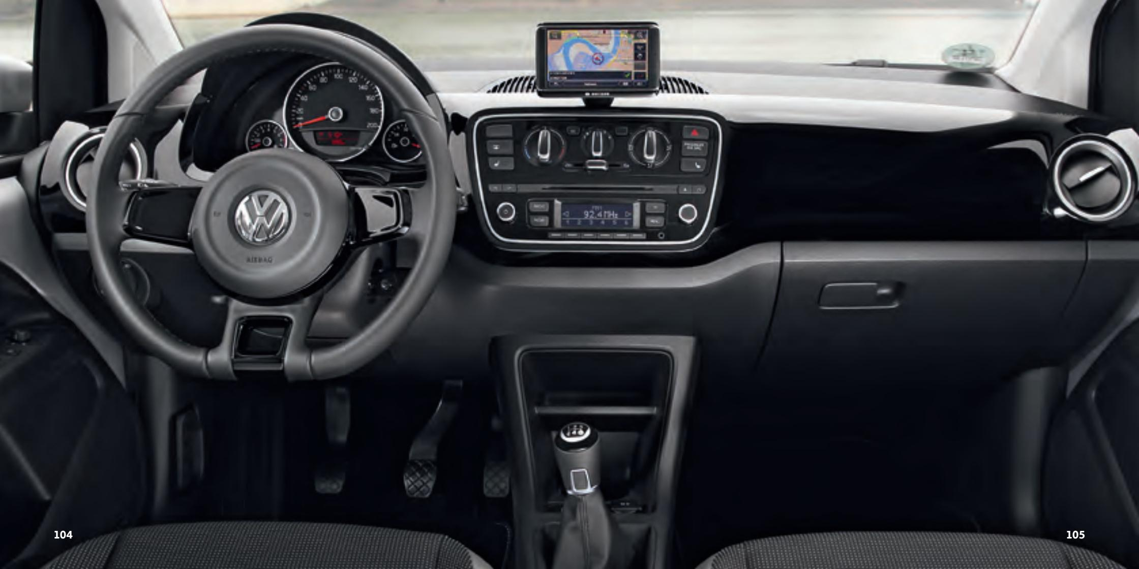
instruments and one digital display. In the move up! and high up!, for example, the largest of the three round analogue instruments is the speedometer in the centre with the integrated digital multifunction display that is an optional feature here. The multifunction display also displays information relating to City Emergency Braking and operational information of the Stop/Start system. To the left of the speedometer there is the tachometer, and to its right is the fuel gauge.
