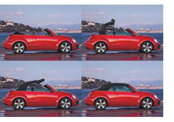
protection system shoots up behind the rear headrests. This mechanism is controlled by the central airbag actuating unit. For the newest version of this rollover protection system, use of high tensile strength steel and aluminium have made it possible to reduce the weight by nearly 50 per cent in comparison to other solutions.
