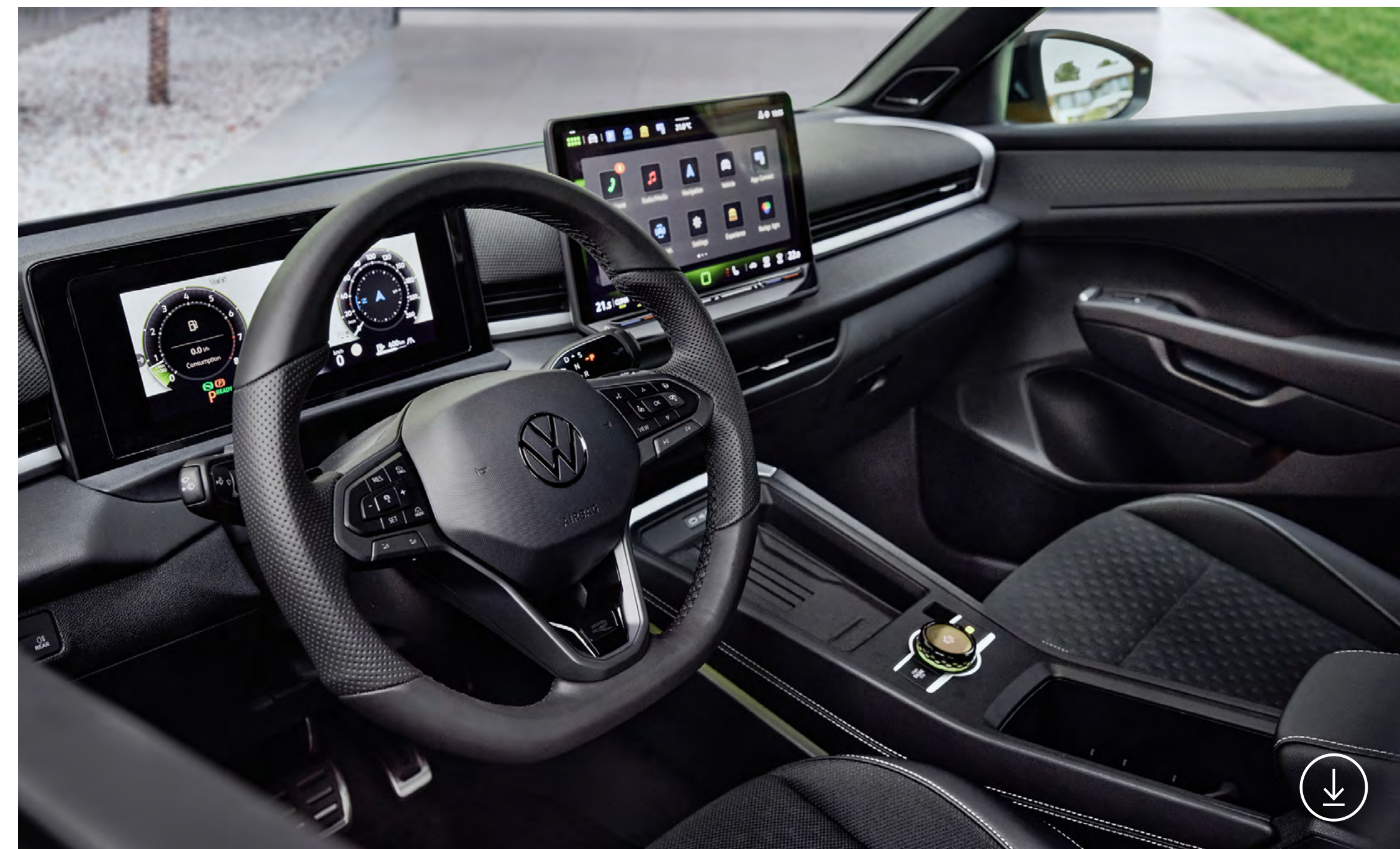
Interior with multifunction steering wheel, digital instruments, infotainment system and driving experience control
