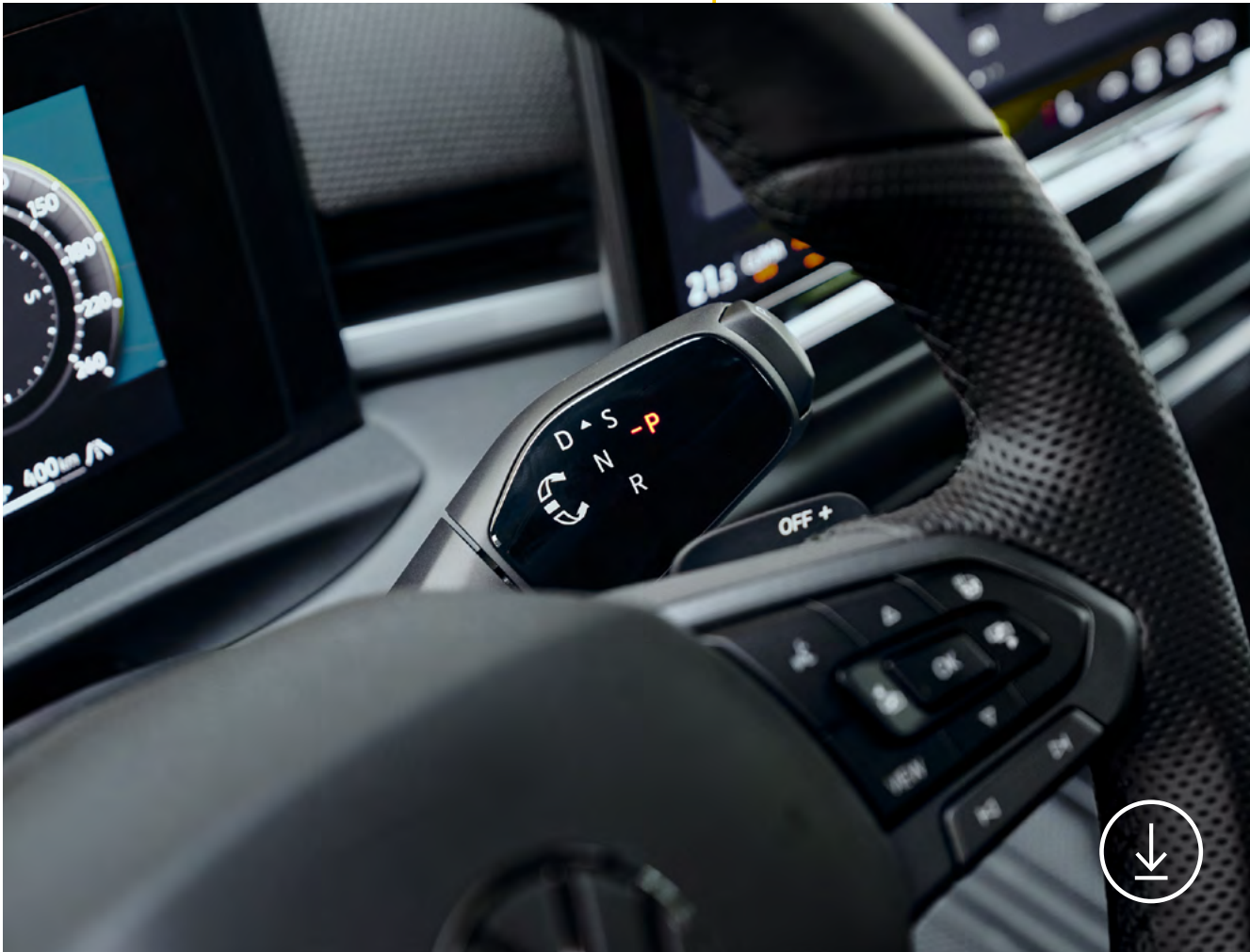
Direct shift gearbox gear lever on the steering column
