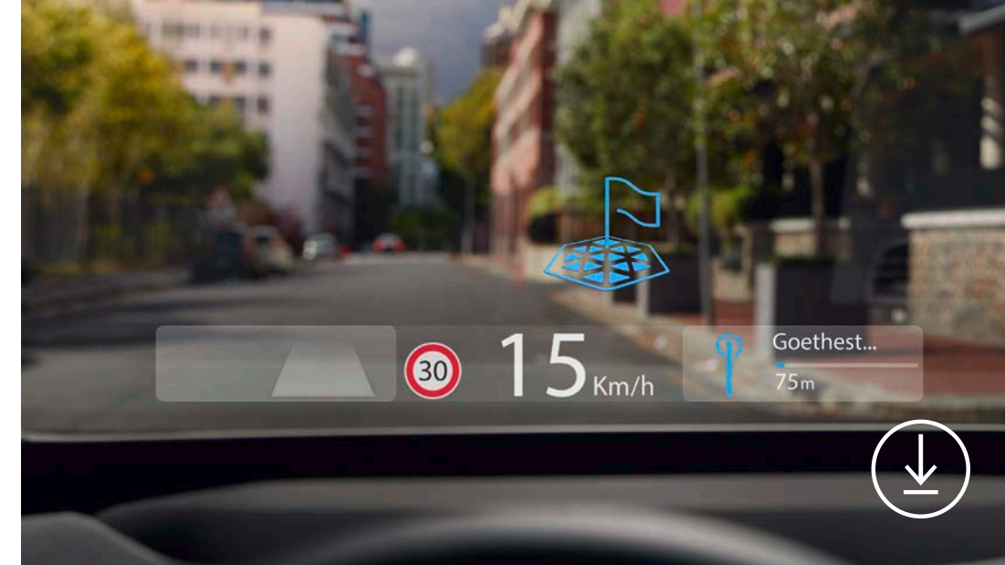
Information on the AR head-up display appears to be ten metres ahead of the vehicle.
