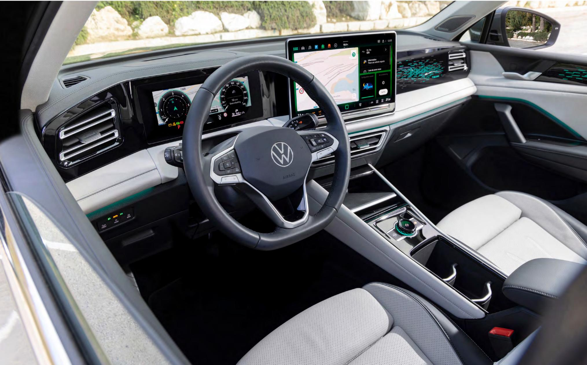
The new interior with 15-inch touch display and Discover Pro Max navigation system
