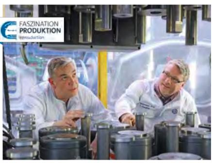
Everything in order: Machinists Volker Matzner (left) and Tino Sandner check the sensors on the press fingerprint tool at the beginning of the measurement process.
