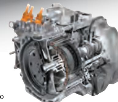
Six-speed dual-clutch gearbox.
