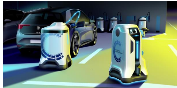
The mobile energy storage device stays with the car* during the charging process. The robot uses this time to charge other electric vehicles.
