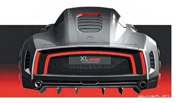
emphasise the width of the XL Sport. Fourth, there is a black diffuser that merges almost seamlessly into the completely enclosed underbody and is finished at each side with a chrome exhaust tailpipe.
