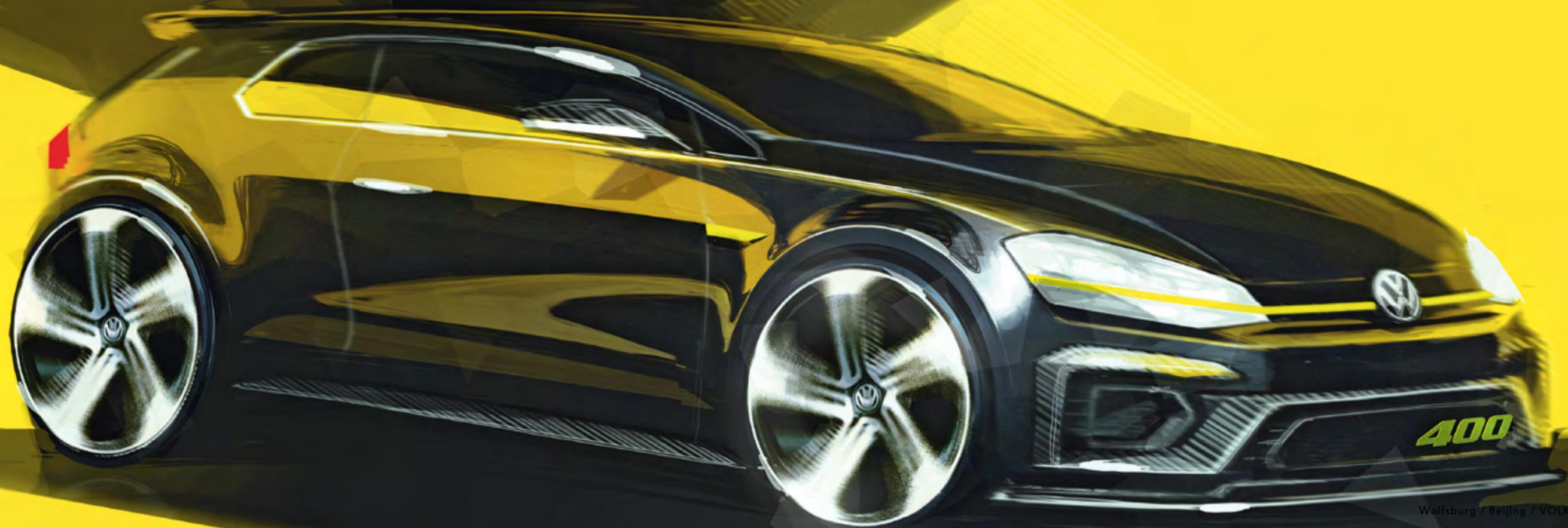
also adapted the side sills to the new contours, creating a uniform transition to the newly designed wheel arches.
