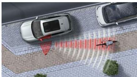
**If another road user is approaching from behind as an occupant is exiting the vehicle, the exit warning system can issue warnings in various stages.**
