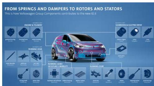
Volkswagen Group Components supplies many parts and components to Zwickau for the manufacture of the ID.3: from the front and rear axles, steering system, brakes and battery system to the complete electric drive.
