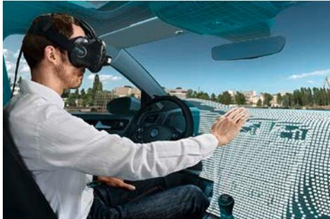
The specialists from the Group IT's Virtual Engineering Lab are working towards the next goal of the virtual concept car. A system of pressure-sensitive pins simulates all the shapes of the interior. This will allow the user to feel the surfaces and controls. Frantisek Zapletal is testing the current version.
