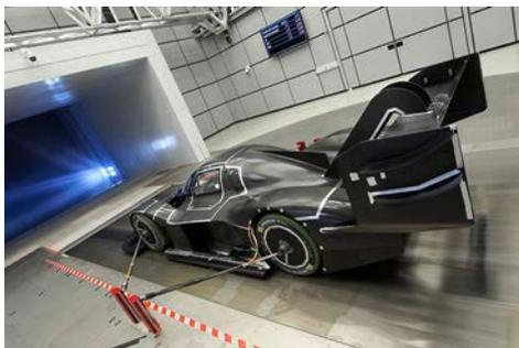
The I.D. R Pikes Peak during aerodynamic tests in the wind tunnel.
