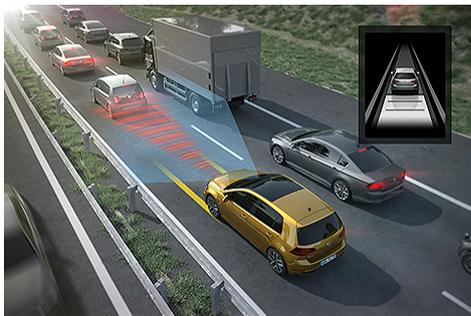
Automatic braking, acceleration and steering in traffic jams
