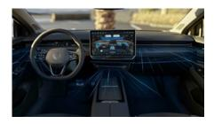
The smart air vents are controlled electronically and move dynamically to distribute the air quickly throughout the interior.
