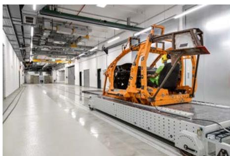
With a run-up of 140 metres the sled can be accelerated to up to 100 km/h.
