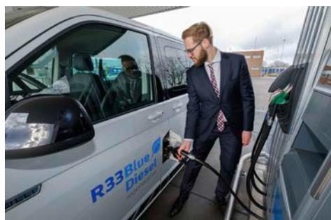
Volkswagen employees tested the new fuel initially. Over a period of nine months, they filled up company vehicles with R33 BlueDiesel only. Up to one third of the new fuel consists of renewable fuel components.
