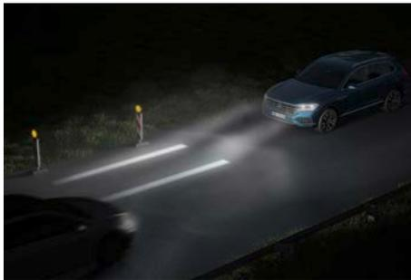
HD LCD headlights allow new light-based assist systems such as “Optical Lane Assist” to be developed. The system projects lane markings onto the road, giving the driver a better idea of the vehicle width when driving through road works, for example.
