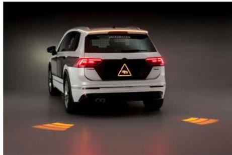
Research vehicle<sup>1)</sup> with exterior HMI: information and warnings to other road users via LC-displays, integrated in in the doors as well as the front and rear ends.
