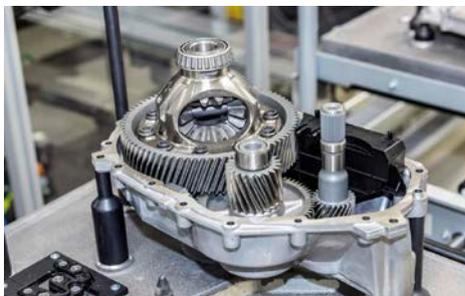
Small shifting unit: the 1-speed gearbox
