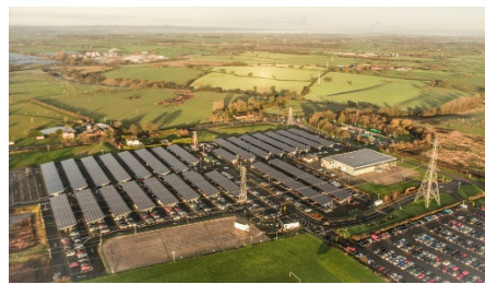
Employee Parking Lots with Solar Roofs at Bentley Motors in Crewe, England
