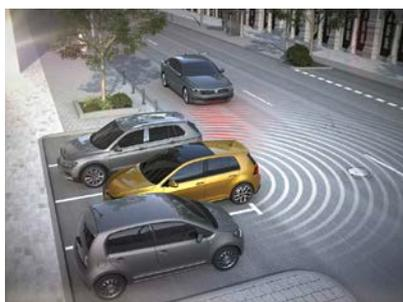
Radar sensors monitor the zone behind the car
