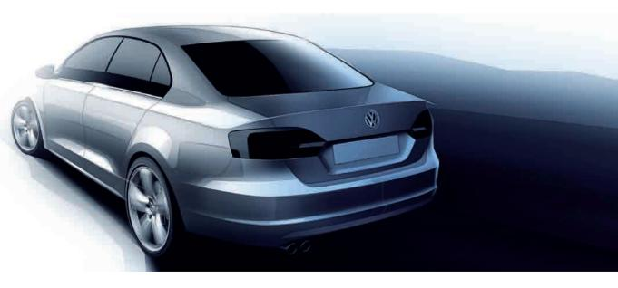
The best example of this: the so-called character or "tornado" line. Its form intersects the main volume of the large, harmonised surfaces, thereby conveying a strong dynamic. The door mirrors also have a sporty appeal: Their design with integrated turn indicators in the form of narrow stripes follows a stylistic solution also implemented in the new Passat and Eos.
