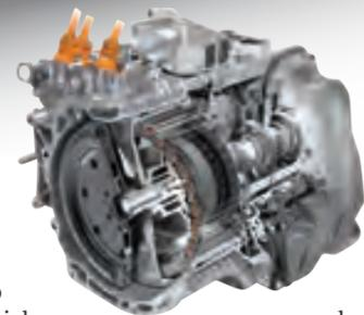
Six-speed dual-clutch gearbox.
