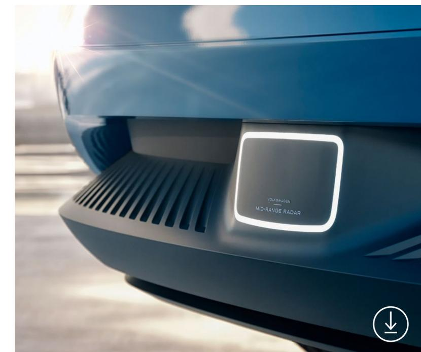
The mid-range radar is illuminated in Level 4 mode
