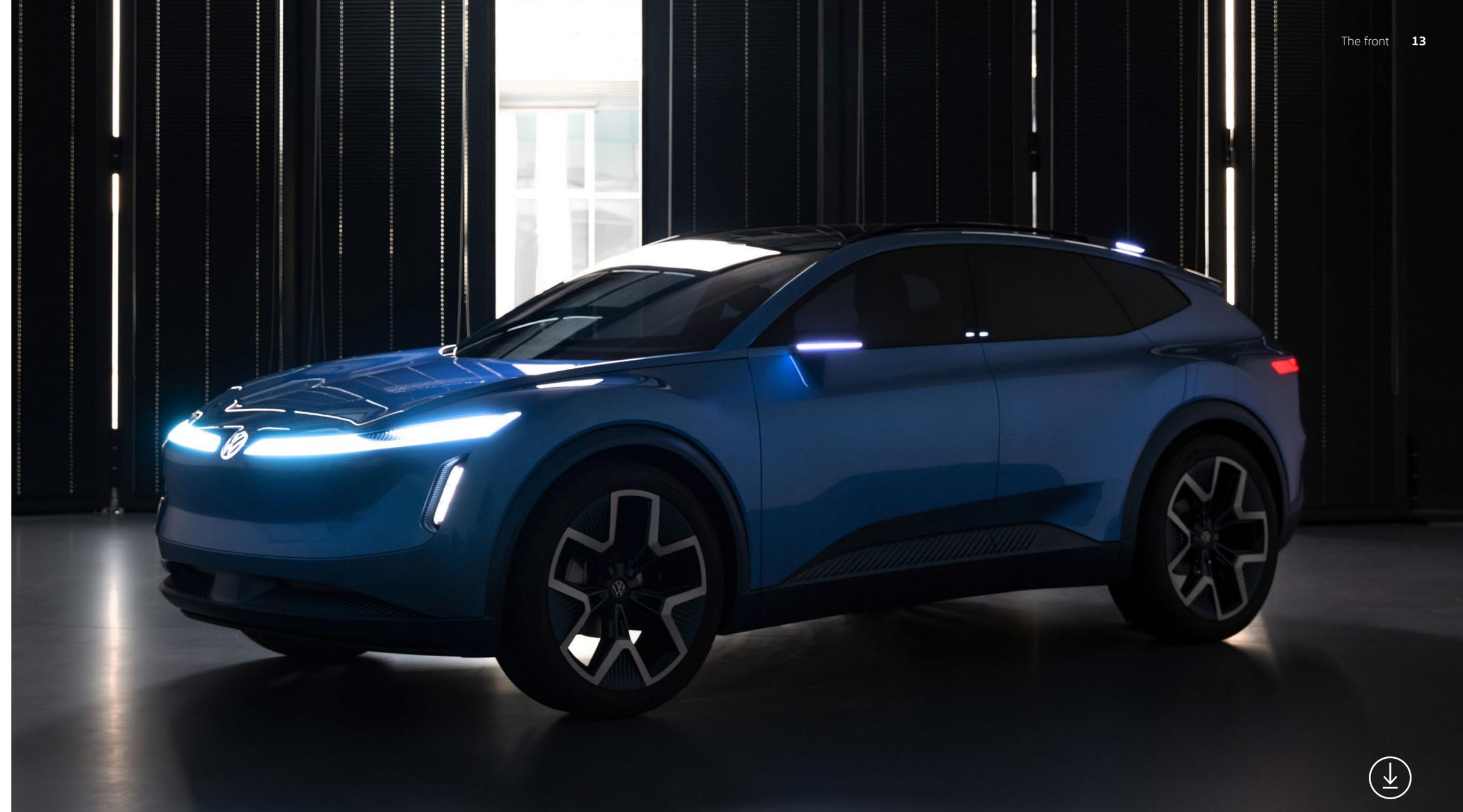
The Light Cloud and the 3D Eyes are responsible for communication; the actual headlights are located on the outside in the bumper
